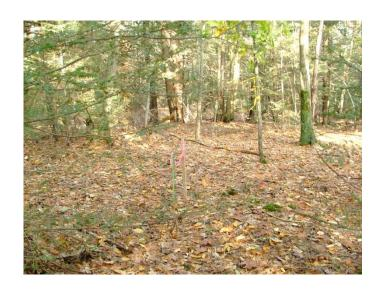
G2. Pin from previous survey (not Eaton Associates). (possibly line between Roberts and Peuschell properties). This pins is shown in Eaton Associates survey as 7.6 feet east of their survey line.
