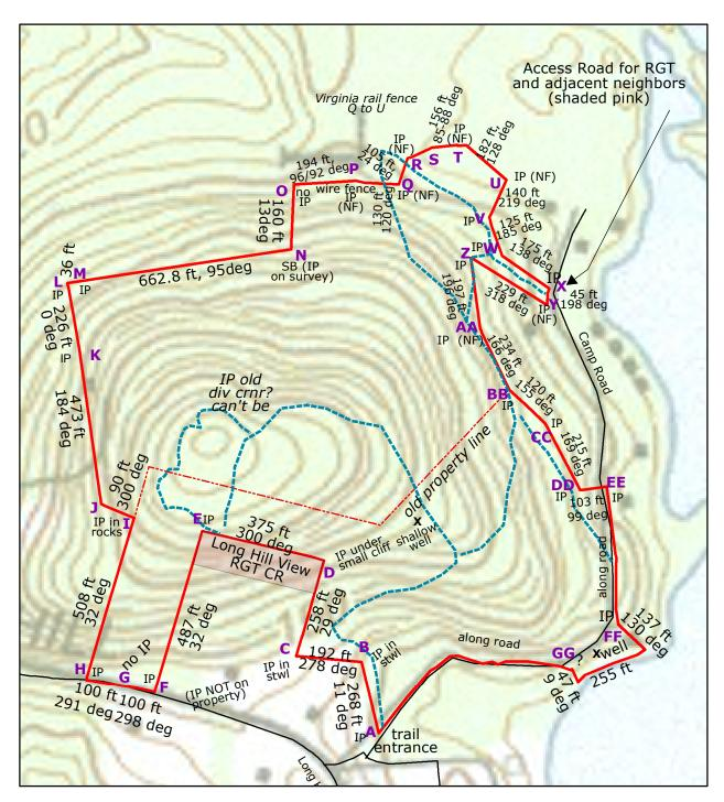
A-EE corner-names used in boundary list (excel) photo list (word) and Nov 2012 annotated surveys and uannotated deed 2836, p.218
